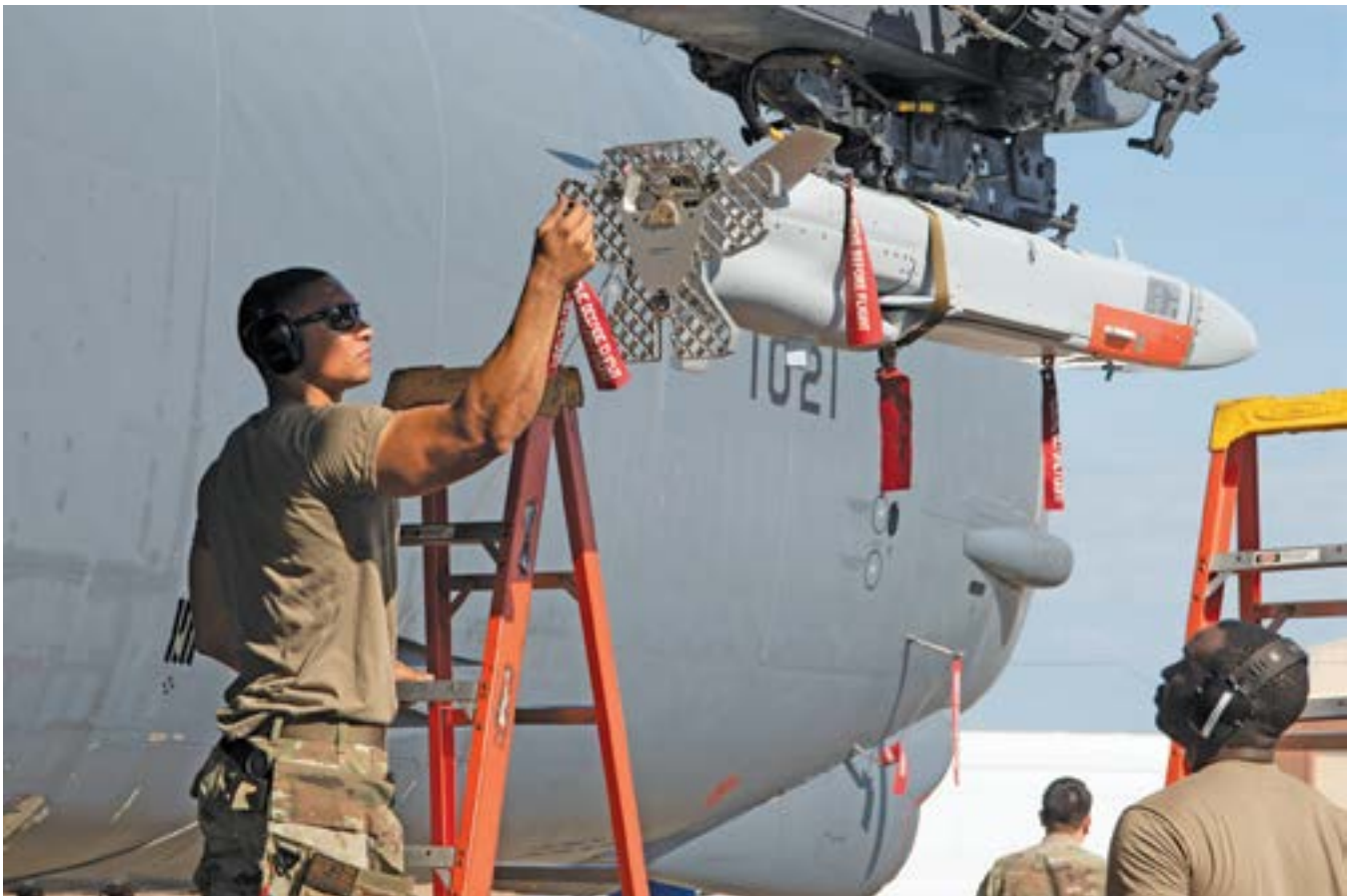
TSgt Skyler McCloyn loads a Miniature Air-Launched Decoy (MALD) ADM 160X onto a B-52 Stratofortress July 13, 2020 at Barksdale AFB, Louisiana. MALD's electronic warfare capabilities are useful in Suppression of Enemy Air Defense (SEAD) operations. Photo by A1C Celeste Zuniga, USAF.
