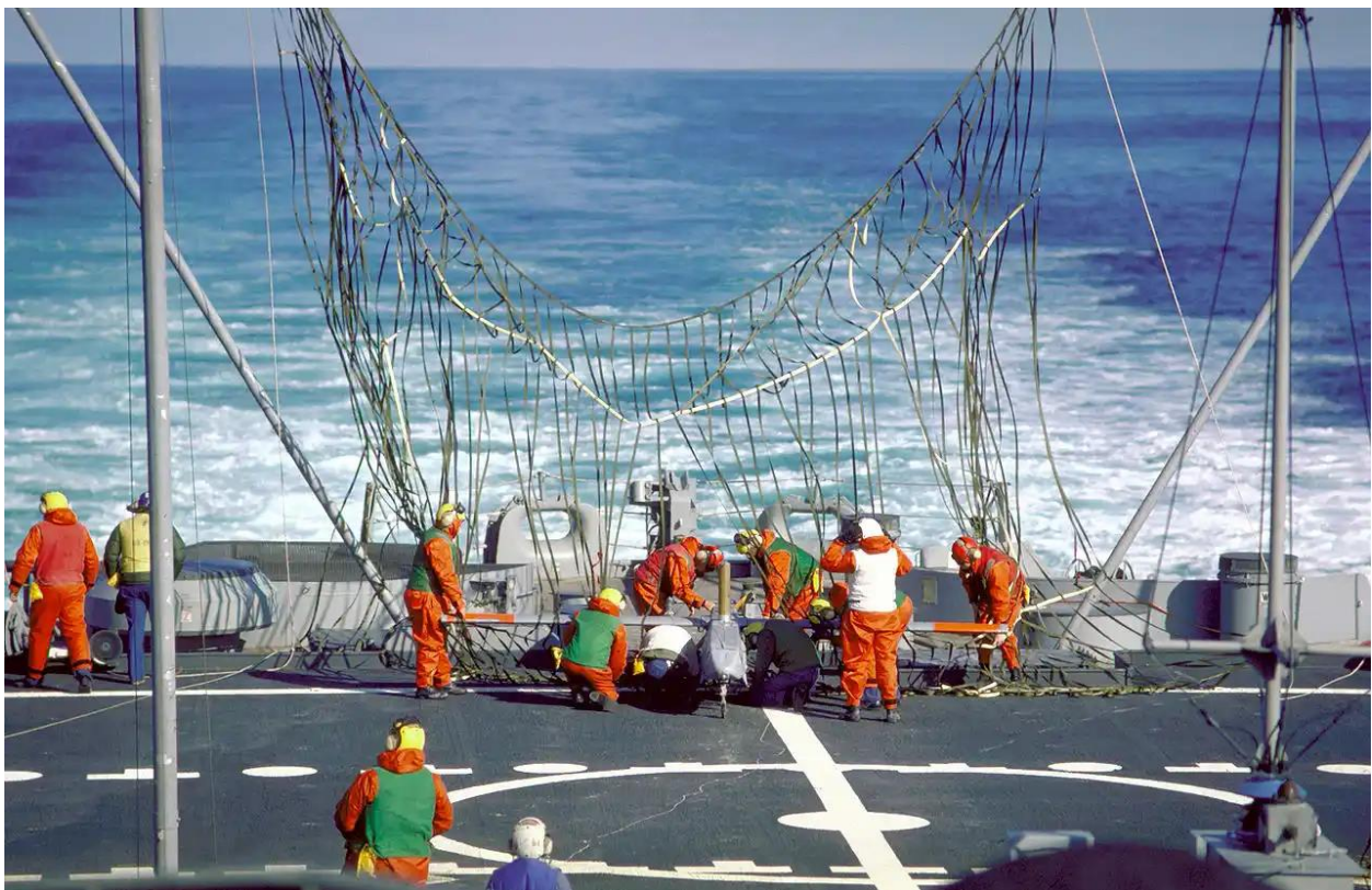
Crewmen disengage a Pioneer I remotely-piloted vehicle (RPV) from a recovery net erected on the stern of the battleship USS IOWA (BB-61) on 1 Nov 1986 (Photo by: PHC Jeff Hilton, USN)
