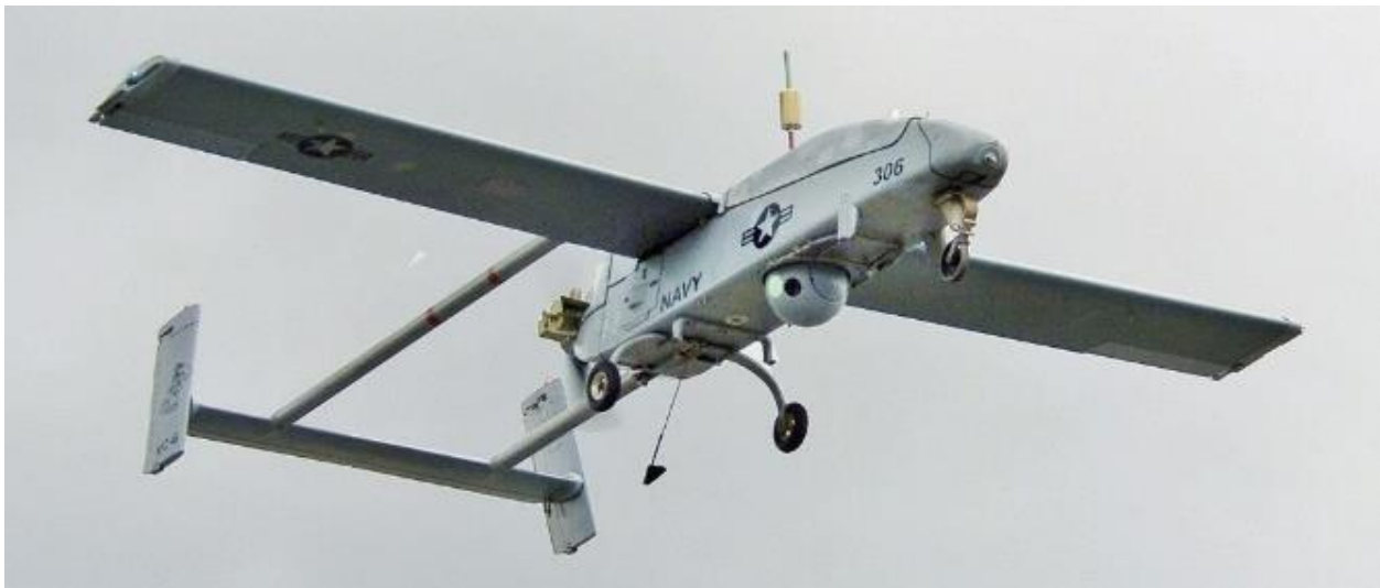
An U.S. Navy RQ-2B Pioneer Unmanned Aerial Vehicle, assigned to the VC-6) uses its sensor turret to scan at the Webster Field Annex of Naval Air Station Patuxent River, Maryland. 2005 (Photo by: Mate 2nd Class Daniel J. McLain, USN)
