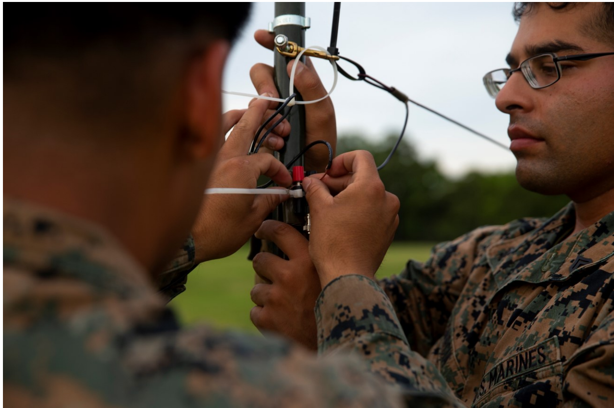
U.S. Marines transmissions system operators with 10th Marine Regiment, 2d Marine Division (MARDIV), set up a Dipole antenna as part of the 2d MARDIV High-Frequency (HF) Competition at Camp Pendleton, Va., July 13, 2021. The competition enhanced HF transmission proficiency and capabilities to prepare Marines for future expeditionary conflicts where the area is either contested or degraded. (U.S. Marine Corps photo by Pfc. Sarah Pyscher)
